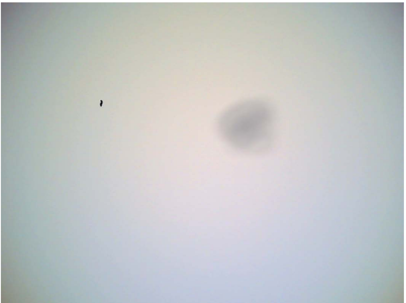
Figure 63 Effects of dust on optical path
