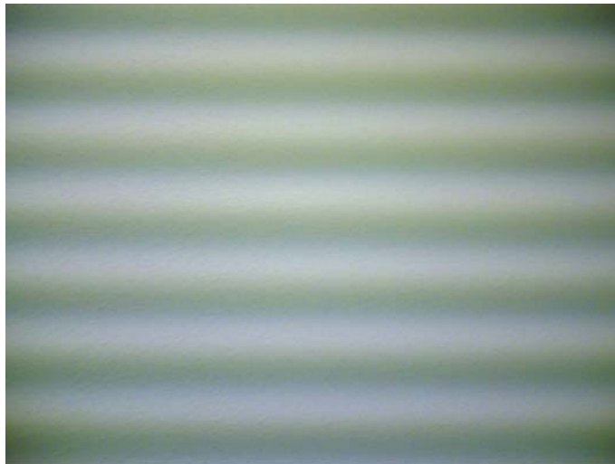
Figure 57 Flicker in an image; object illuminated by strong fluorescent light
