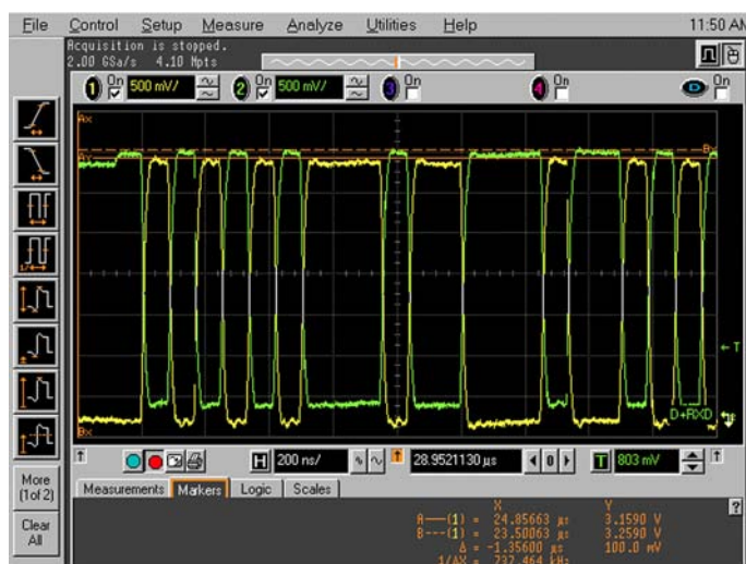
Figure 46 USB 1: D-TXD (PopPort TM™ pin 6) and D+RXD (PopPort TM™ pin 7) voltage levels when USB is connected.
