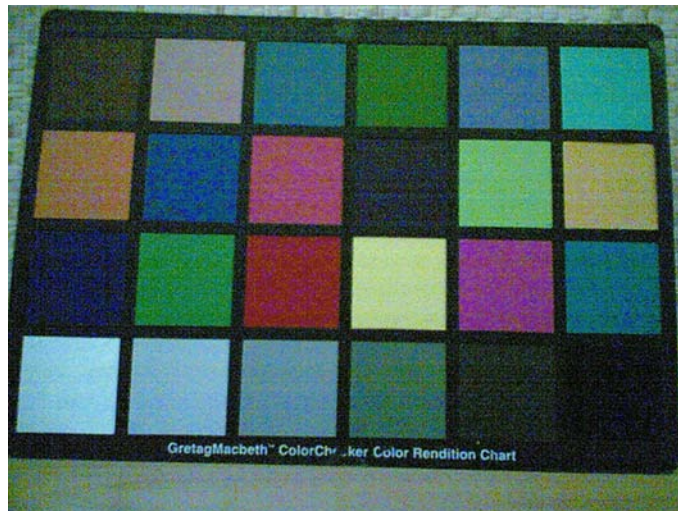
Figure 55 Noisy image taken in +70 degrees Celsius
