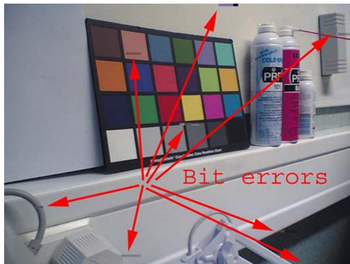
Figure 66 Bit errors caused by JPEG compression
