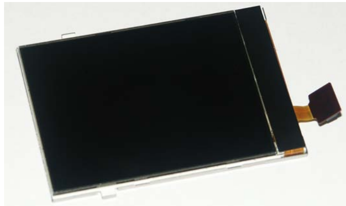
Figure 91 General diagram of the LCD module
